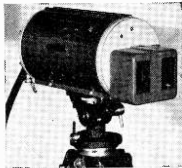
Stereoscopic television camera showing optical system for producing left- and right-eye views (Pye).
